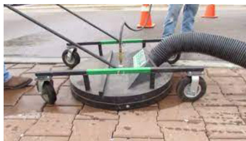
PaveDrain Vac Head for Cleaning
