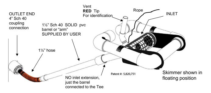
2. Glue the  $1\frac{1}{2}$ " Sch 40 **barrel** pipe to the  $1\frac{1}{2}$ " white coupling on the **hose**.
