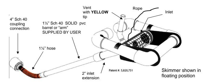
2. Glue the 6' long 1<sup>1</sup>/<sub>2</sub>" sch 40 **barrel** to the 1<sup>1</sup>/<sub>2</sub>" grey coupling on the **hose**.
