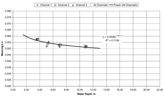
Manning's n vs. Water Depth FLEXAMAT (Tested with 30% Bottom Slope Gradient)
