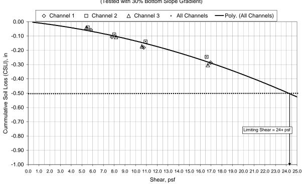
Limiting Shear via ASTM D 6460 FLEXAMAT (Tested with 30% Bottom Slope Gradient)
