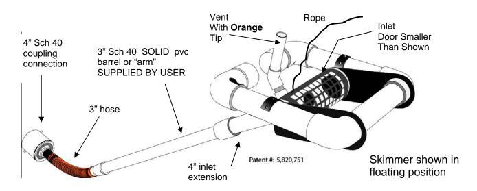
2. Glue the 8' long 3" sch 40 barrel to the 3" grey coupling on the hose.
