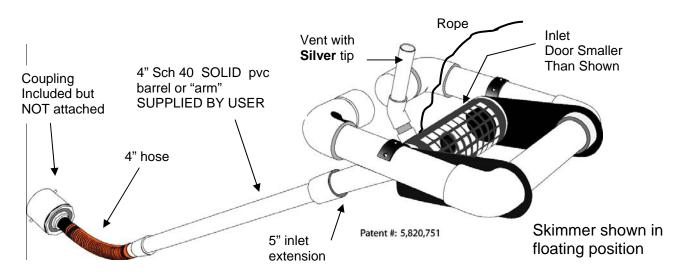
2. Glue the 8' long 4" sch 40 barrel to the 4" grey coupling on the hose.
