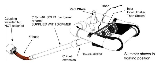
2. Glue the 10' long 5" sch 40 **barrel** to the 5" white coupling on the **hose**.
