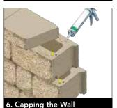
Clean off the last course of Keystone Century Wall in preparation for the cap or coping to finalize the wall. With units dry and clean, use a construction adhesive for a mechanical bond. Install capping units, architectural precast concrete, or cut stone as a coping element. Cap may be flush or overhanging as required by aesthetics and
