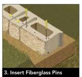
Place the shouldered fiberglass pins into the appropriate holes to achieve the desired setback position of the Keystone Century Wall units. Place pins in the front hole(s) for near vertical alignment. Place pins in the rear holes for an 8° setback per course.
