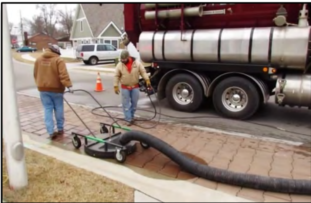
Combination Sewer Truck with 1,500 gallon water tank
