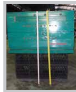
Creep testing on the Heavy Duty R-Tank (5-Plate) was done using four Double R-Tanks, also unconfined.
