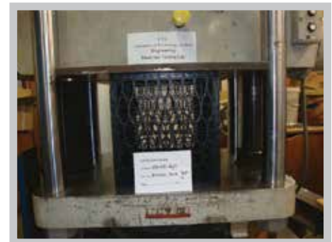
Unconfined Compression Test
