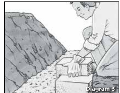
Construction of the next course
