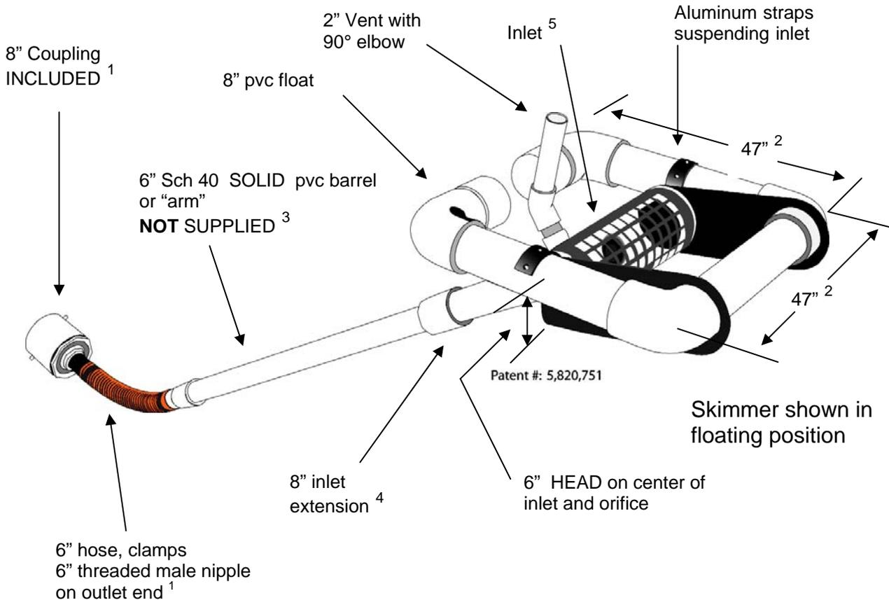
1. Hose can be attached to outlet using the threaded 6" nipple. Typical methods used: on a metal structure a steel stubout welded on the side at the bottom with a 6" threaded coupling or reducers; on a concrete structure with a hole or orifice at the bottom, use a steel plate with a hole and coupling welded to it that will fit over the hole in the concrete and bolted to the structure with sealant.
