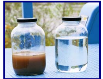
Discharge from sand filter: 10 NTU
