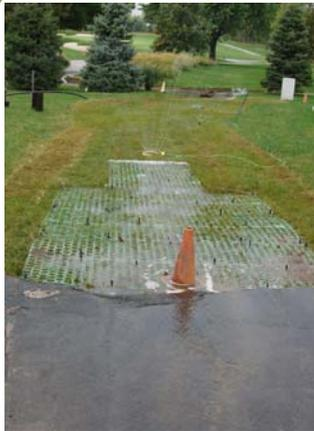
Vegetated drainage way able to exceed 15 lbs/ft<sup>2</sup> shear stress.
