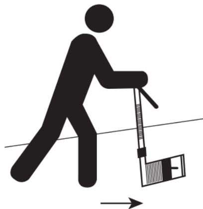
and dependable solution to erosion control blanket installation and sod laying in sloped areas. The Staple Wasp is constructed of lightweight and durable material.
