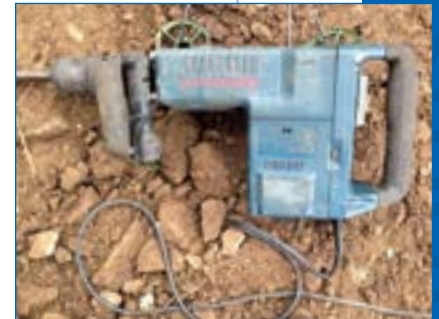
1 A Bosch Hammer can be used for extremely dense and/or rocky soils.
