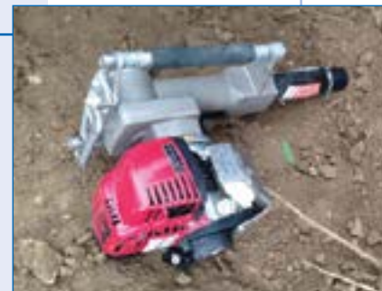
2 A lightweight hand operated gas hammer is very operator friendly.
