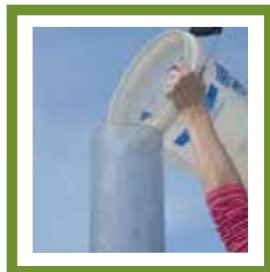
Figure 9: Filling Infiltrometer with Water
