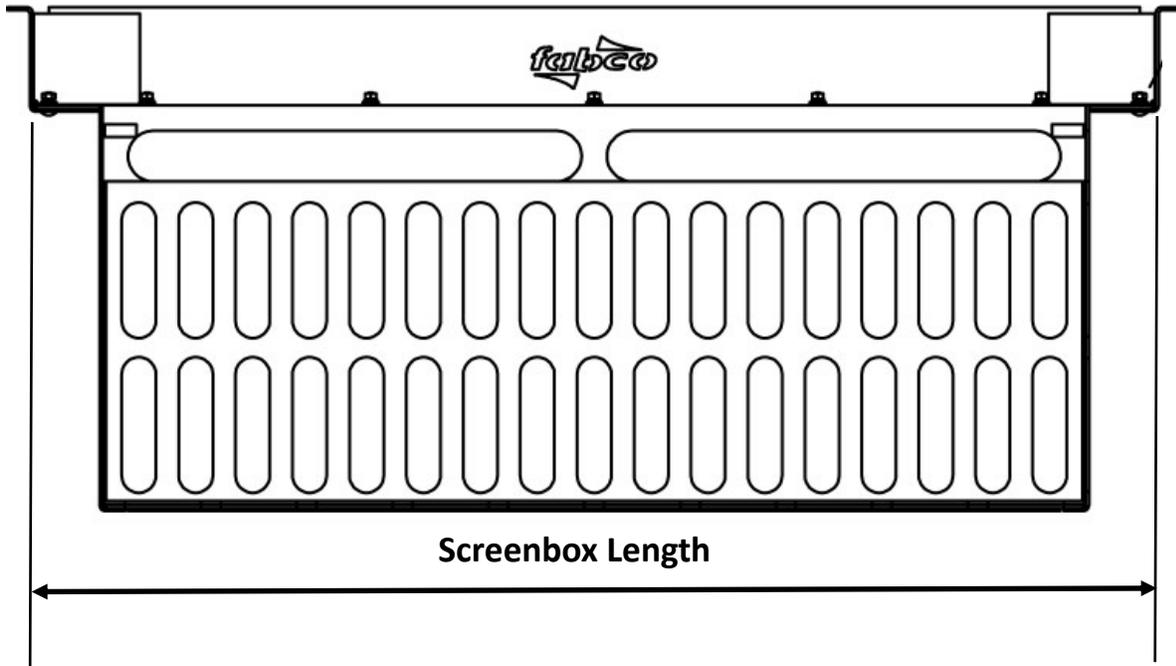
**Sliding Flanges should be set at the grate frame clear space measurements**
