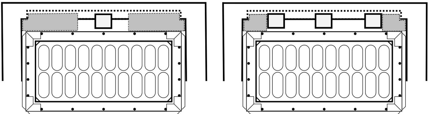
The SplashGuards are cut down to fit the curb throat opening as shown above. Please note that the intent of the SplashGuard is to divert the flow down the curbline into the StormSack BMP unit.
